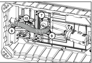
To install the chip-removal system, turn the Foreman onto one side and from the inside of the machine base (3), insert the vacuum port (5) into the hole in the back of the base and secure it from the outside with two self-tapping screws (6). Fasten the vacuum shroud (7) to the machine with four truss-head machine screws (8).
