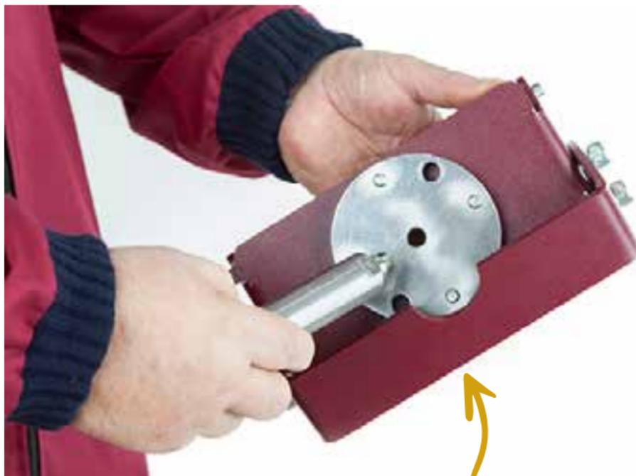
Turn the **SteadyPro** over to access the stem fitting location
