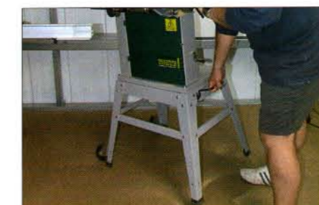
▲ Pic 11: Built-in wheels allow you to store the saw out of the way
