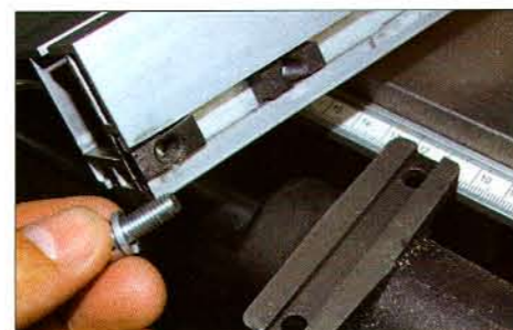
▲ Pic 5: You can see where the small cast brackets have split preventing the fence from locking properly to the casting
