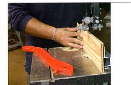
▲ Pic 10: Deep ripping wasn't a problem, and once the fence problem was rectified the saw would make veneer rips easily
