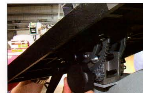
▲ Pic 9: Tilting the table is a one handed operation; the small knob above micro-adjusts the thrust roller
