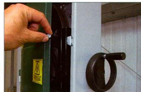
▲ Pic 6: Although micro-switched, new legislation means that the doors require a tool to open them
