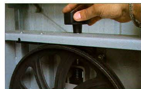
▲ Pic 2: This knob sets the blade tension; the spring is pretty substantial
