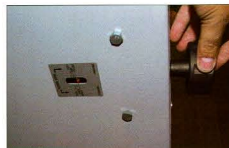
▲ Pic 3: The tension can be read at the back of the saw, the scale indicating blade width
