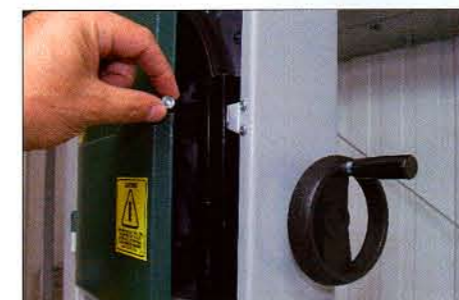
▲ Pic 7: Top side adjusters are micro-adjustable; the thrust roller needs a hex' key
