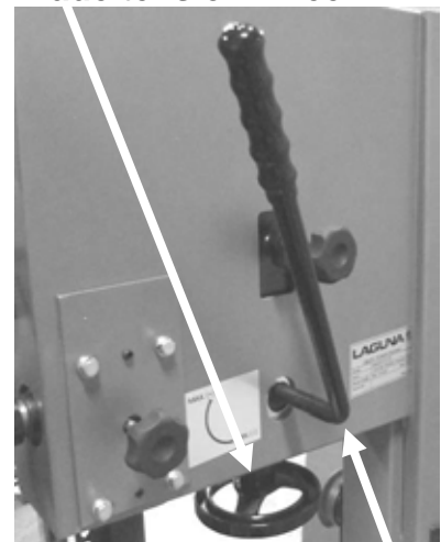
Quick action blade tension lever (activated)
