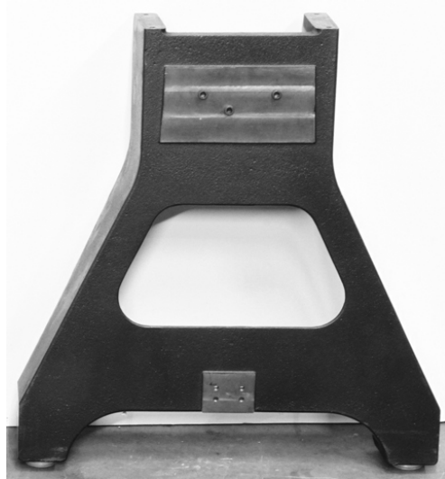
Legs with adjustable feet assembled
