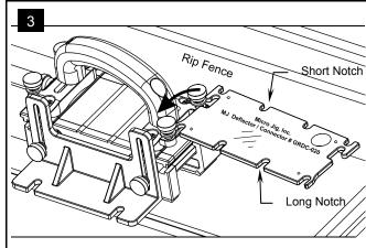
**Step 3:** Position the Deflector/Connector (D/C) as shown in Drawing 3 with the flat smooth surface facing up. Slide the D/C from the right side of the GRR-Ripper® with the two notches engaged onto the nylon shoulder washers (P). Push the D/C until the Nylon Shoulder Washers (P) are fully seated in the notches. Finger tighten the thumb screws (T). The D/C is now ready for ripping on the table saw (see Drawing 4).
