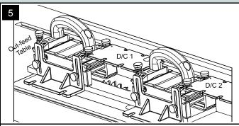
↑ One D/C connects two GRR-Rippers® fore and aft, while a second D/C serves as a deflector. An out-feed table is necessary with this configuration! Use of the MJ Splitter is recommended with this setup.
