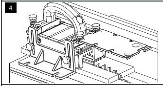
↑ One D/C is used as a chip deflector and blade cover on a single GRR-Ripper® operation on table saw. This setup can also be used with the leap-frogging technique, but do not lift off the GRR-Ripper® with the D/C attached in this position at an excessive angle.
