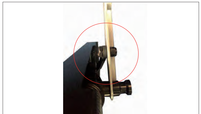
Step 20: Secure the Octagon drum lid to the cyclone funnel using hex bolts (8) 8 mm*19 mm, flat washers (16) 8 mm*OD18*2T and hex nuts (8) 8 mm. Make sure to first attach all the bolts on before tightening the bolts.
