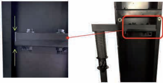
Step 14: Secure the base of the foot pedal bar to the triangular support plate by holding the lower support plate vertically up against the foot pedal bar and secure the U channel onto the foot pedal bar using (2) 5/16"x1-3/4" hex bolts, (4) 5/16" x 18 x 2 flat washers and (2) 5/16" hex nuts from the inside out. Follow the same steps for the opposite side.
