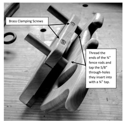
Do not mount the adjustable fence rods yet (easier to finish everything without the rods in the way).
