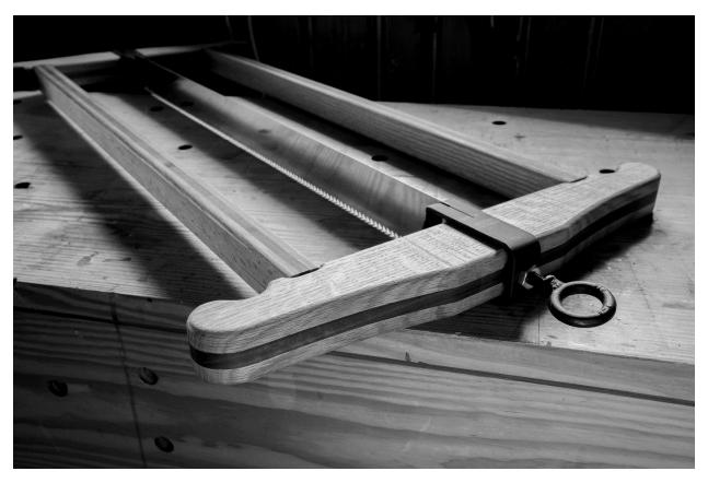
• Now close the brass hex nut to within 1/16" away from bracket surface. Hold frame saw assembly upright, and using a stout screwdriver, give the eyebolt a 180-degree turn clockwise. By now the brass
