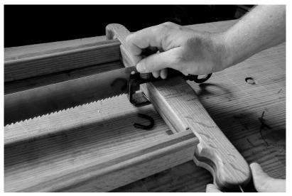
striker plate is oriented toward the eyebolt, which keeps the eyebolt from walking under tension. Reassemble the bracket in place.
