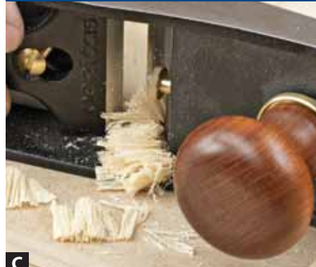
C This plane's iron, sharpened to a mirror polish with an 8,000-grit stone, yields shaved ribbons when cutting end-grain pine.
