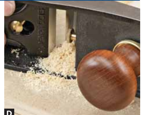
D Sharpened only to 1,000 grit, this plane leaves crumb-like shavings and torn-out grain in its wake. Two more grits would improve this cut.
