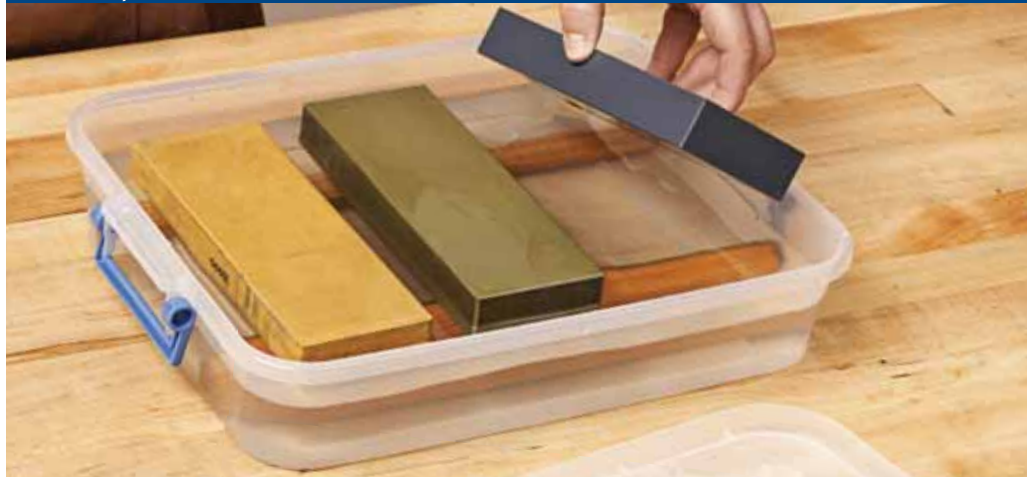
Water stones must soak 15 minutes before use. We store them on maple strips in an $8 plastic cake carrier.
