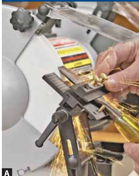
Grind a primary bevel angle onto chisels and plane irons with cool-cutting aluminum oxide wheels and a tool rest to maintain a consistent angle.
