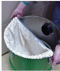
Drum filter removal
