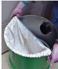
Drum filter removal
