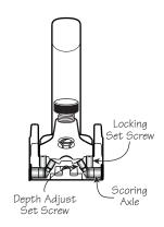
Figure 4: Setting the scoring blade.
