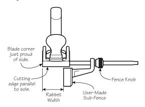
Figure 3: Setting the blade and fence.
