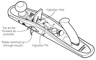
Figure 2: Installing the blade.
