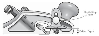
Figure 5: Setting the depth stop.
