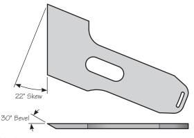
Figure 8: Blade geometry.
