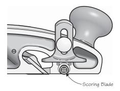
Figure 6: Setting the scoring blade.
