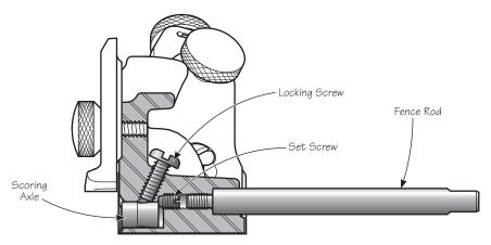
Figure 7: Scoring blade position.
