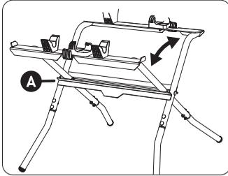
1. Fully unfold stand. Always use on solid level ground. The stand is fully opened when the center cross brackets (A) will not allow the stand to unfold any further.
