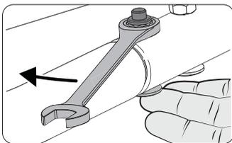
4. Thread the eight lock nuts onto the carriage bolts, and then tighten. Leave the two on the right rear leg loose (marked with a label).
