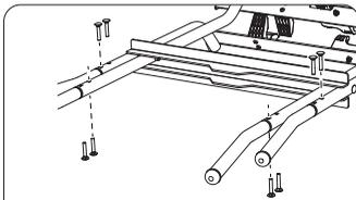
3. Insert carriage bolts through the holes in the legs.
