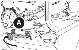
3. Always orient the front of the saw to the front of the stand. Always make sure the clamps (A) (B) are locked before using the saw.
