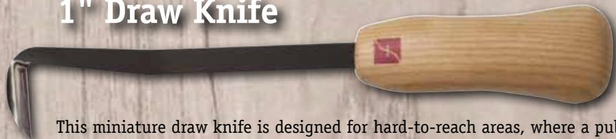
This miniature draw knife is designed for hard-to-reach areas, where a pulling action is more conducive to efficient stock removal. The shank allows the cutting angle to be changed easily for contoured cuts.
