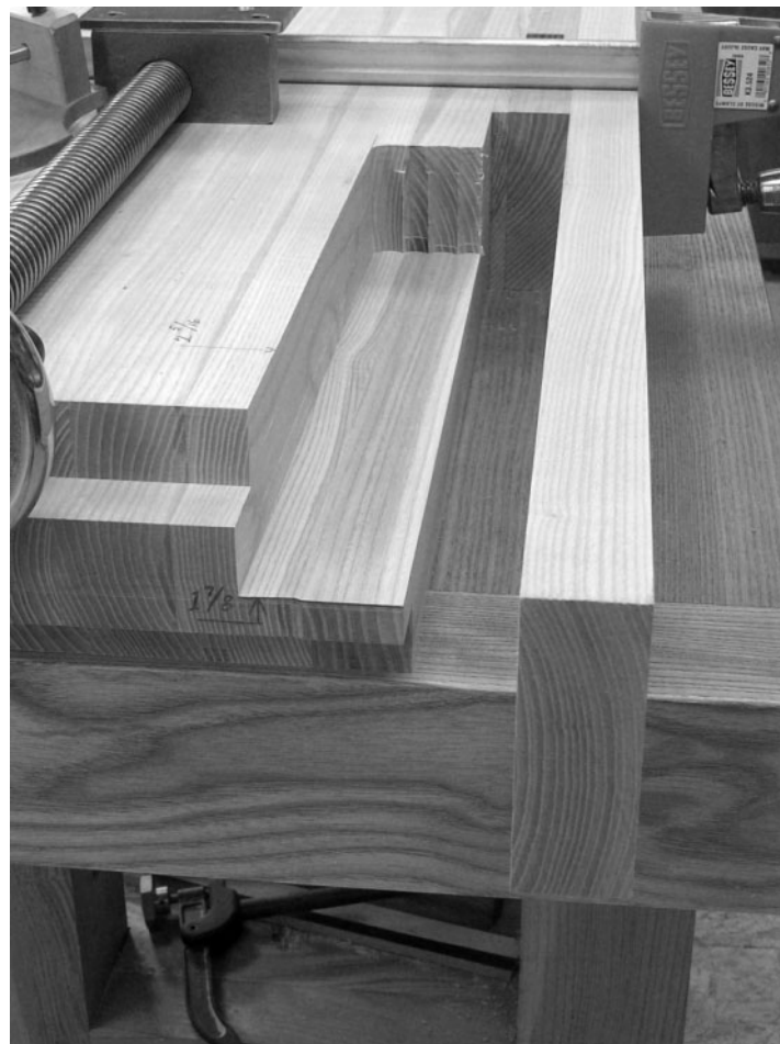
The completed cavity with dog hole strip and front laminate clamped in place.
