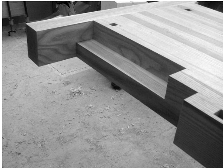
The cavity with end cap and dog hole strip in place.
