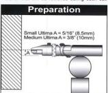
Set the tool rest so that the edge of the cutter is on centre using the dimensions as shown above as a guide.
