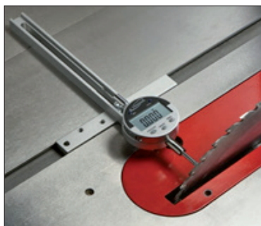
A dedicated saw dial indicator. Such as this one by 'lagging'.
