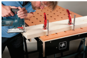
Quick surface clamping using Quick Lever Guide Rail Clamps, code 103061
