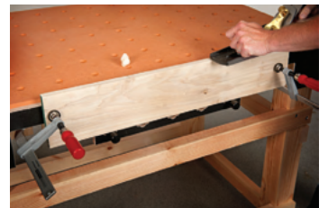
Using dogs and clamps to ensure the work piece is clamped square and level
