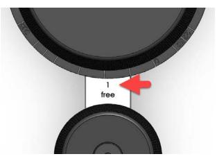
3. Rotate the *Miter Angle Dial* until the desired miter angle is indicated, then re-tighten the *Grip*. The example image below shows a 15° left miter angle.
