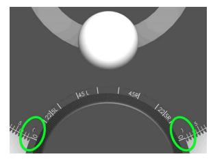
3. After selecting 0°, tighten the *Grip* (A) by rotating it clockwise.
