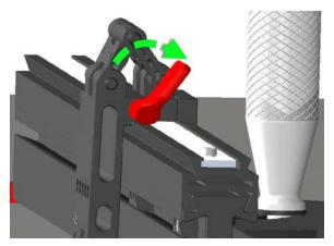
2. Insert a spare *Sliding Wedge* into the slot on the front of the *Fence Assembly* and position it behind the flip stop. Align the center hole of the *Sliding Wedge* (highlighted in blue) with the center hole on the front of the flip stop.
