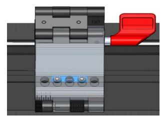
3. Insert the spare *Thumbscrew* into the hole just left of the center hole of the flip stop. Use the hex tip of the *Thumbscrew* to tighten the set screw of the *Sliding Wedge* (highlighted in blue) you placed in Step 2. Turn the *Thumbscrew* clockwise until the set screw is snug.
