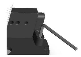
Use a precision square against the side of the miter bar without expansion discs to square the *Vertical Faceplate* as you re-tighten the four *Socket-Head Bolts* you loosened in step 4. Use the included 4mm hex wrench to tighten the bolts.
