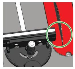
2. Adjust the *Fence Assembly* to the left or right as needed, then tighten the *Thumbscrews* on the back side of the miter gauge body to secure the fence from moving during cutting operations.
