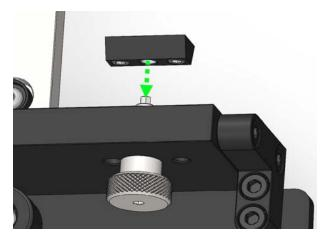
3. Repeat steps 1 and 2 using a second *Thumbscrew* and *Sliding Wedge* as shown.
