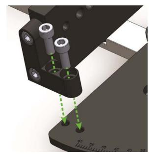
Note that the diameter of the holes in the L brackets are slightly oversized to provide for precise positioning (squaring) of the Vertical Faceplate with the rest of the assembly. To prepare for squaring, loosen the Grip (A) slightly by turning it counter-clockwise.
