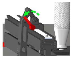
2. Slide the *Flip Stop Assembly* along the top of the *Fence Assembly* extrusion to the desired distance from the blade. Read the built-in ruler on the fence at the edge of the flip stop carrier here.
