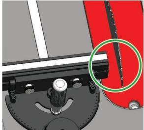
Adjust the Fence Assembly to the left or right as needed, then tighten the Thumbscrews on the back side of the Miter Gauge Body to secure the fence from moving during cutting operations.
