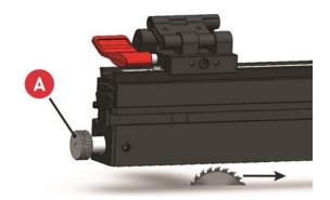
4. Draw the upper portion of the *Fence Assembly* extrusion to the side to extend the fence.
