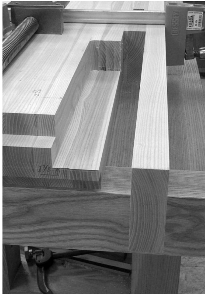
The completed cavity with dog hole strip and front laminate clamped in place.
